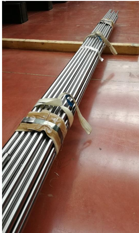
Figura 1: Corretto packaging per barre metalliche/Acceptable packaging for metal bars
